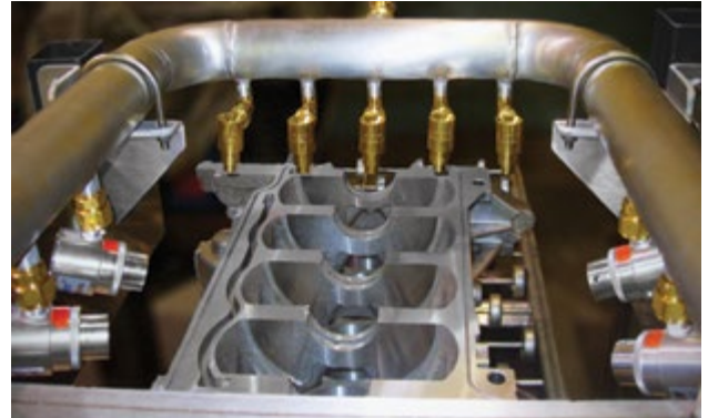
Adjustable Air Amplifiers and High Velocity Air Jets dry an engine block prior to assembly.
