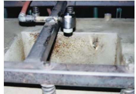
A Model 121021 1-1/4" (32mm) High Temperature Air Amplifier directs hot air to a rotational mold cavity for uniform wall thickness of the plastic part.
