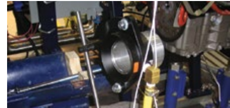
A Model 120024 4" (102mm) Super Air Amplifier cools an engine during dynamometer testing.
